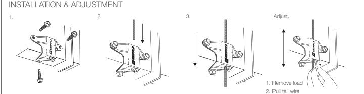
Ensure a minimum 75 mm of tail wire exits the hanger.
