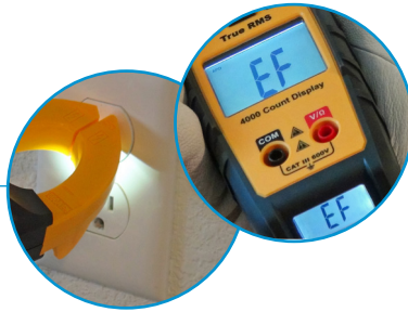
Non-Contact Voltage Tester Screen displays EF (Electromagnetic Field)
