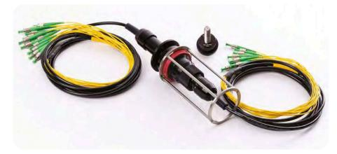
The IRIS system can accommodate up to 12 single-mode or multimode fiber optic channels. For ITS applications, the plug side of IRIS features 6 ft. pigtails with choice of ST, SC, or LC simplex connectors. The receptacle side is purchased with choice of fiber count and length of blunt end.
