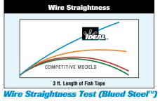
This test was performed by placing each sample of wire on a table such that it was touching two pins that were 3 ft. apart. (A straight edge connected the two pins.) Each sample was pressed toward the straight edge and then slowly released until the wire came to rest at an equilibrium state. The maximum distance from the wire to the straight edge was recorded.
